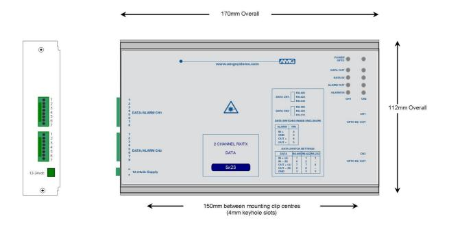
The **AMG5523** is a **DUAL** standalone system which provides two independent channels, each designed to transmit and receive one bi-directional alarm plus one data signal over one Singlemode optical fibre.
